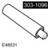
Pilot (spigot) bearing installer/clutch alignment 303-1096
